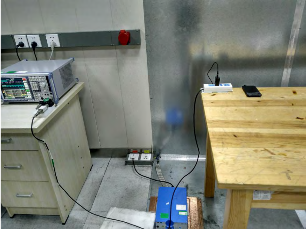
FCC RADIATED EMISSION TEST SETUP
