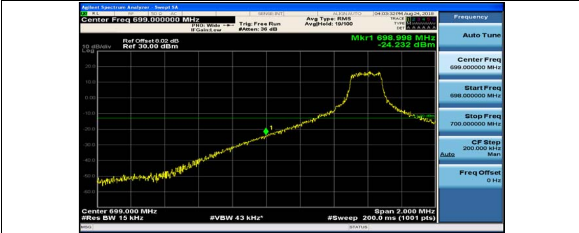
Channel Bandwidth: 10 MHz_LCH_16QAM_1RB#24
