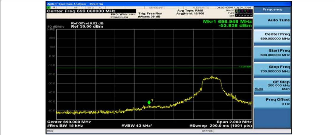
Channel Bandwidth: 10 MHz_LCH_16QAM_25RB#0
