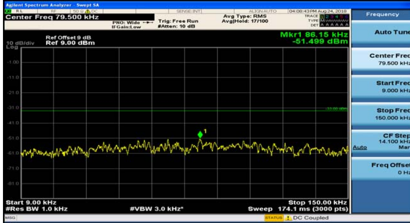
(Channel Bandwidth: 1.4 MHz)_MCH_QPSK_1RB#0
