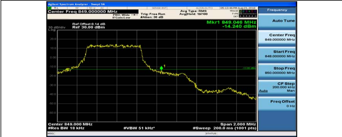
(Channel Bandwidth: 1.4 MHz)_HCH_QPSK_6RB#0
