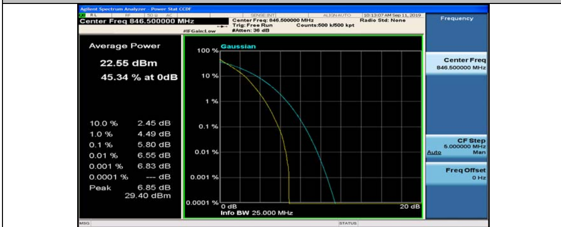
(Channel Bandwidth: 5 MHz)_HCH_QPSK_25RB#0
