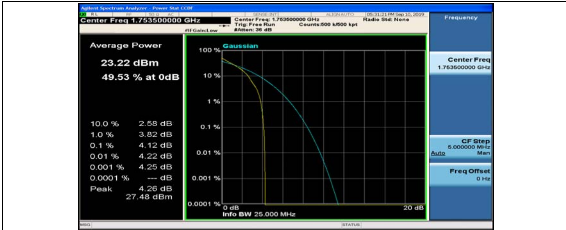
(Channel Bandwidth: 3 MHz)_HCH_QPSK_1RB#14
