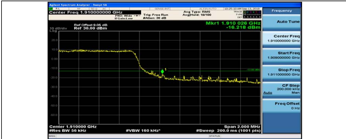
(Channel Bandwidth: 5 MHz)_HCH_QPSK_25RB#0
