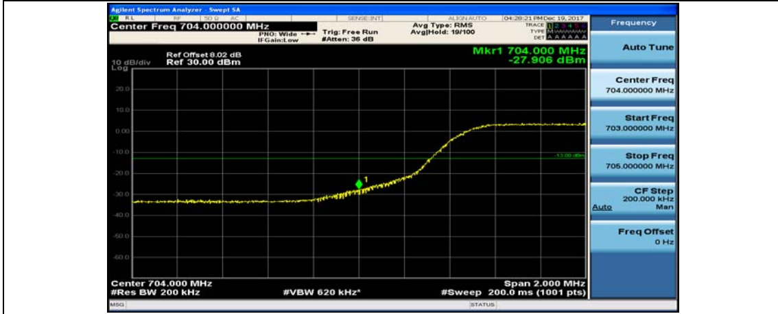
Channel Bandwidth: 10 MHz_HCH_16QAM_1RB#0
