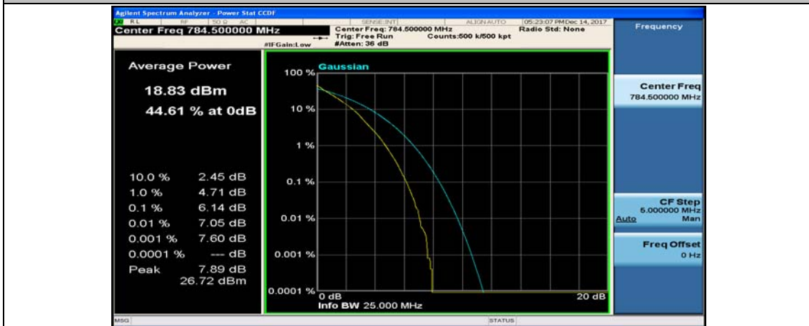
(Channel Bandwidth: 5 MHz)_HCH_QPSK_12RB#6
