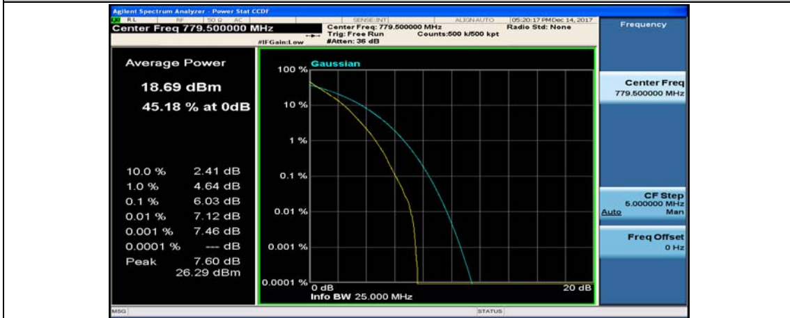
(Channel Bandwidth: 5 MHz)_LCH_QPSK_25RB#0
