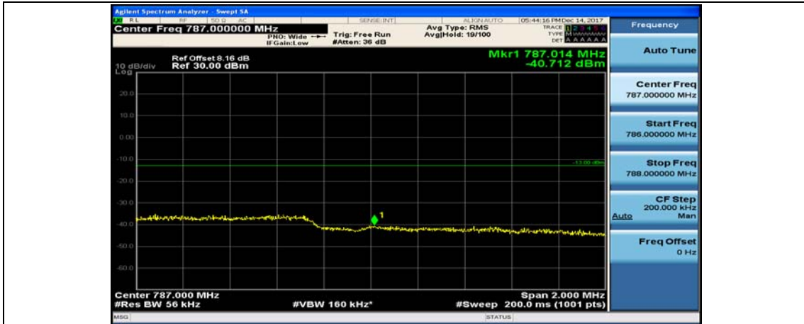
(Channel Bandwidth: 5 MHz)_HCH_16QAM_12RB#6
