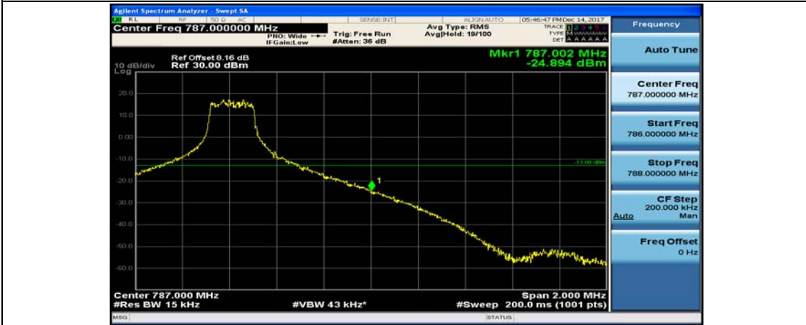
Channel Bandwidth: 10 MHz_HCH_QPSK_25RB#0
