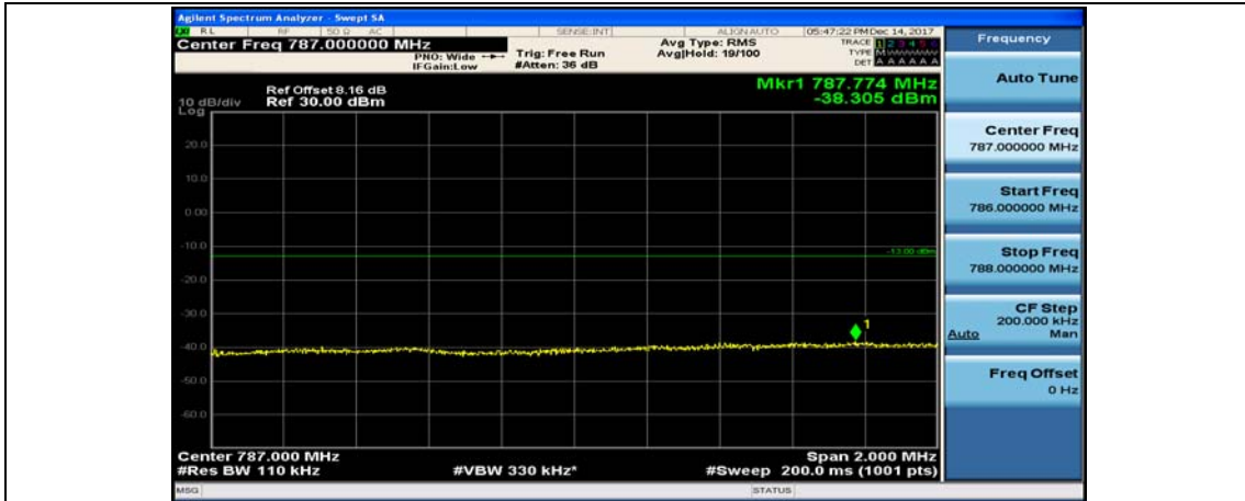
Channel Bandwidth: 10 MHz_HCH_QPSK_25RB#25
