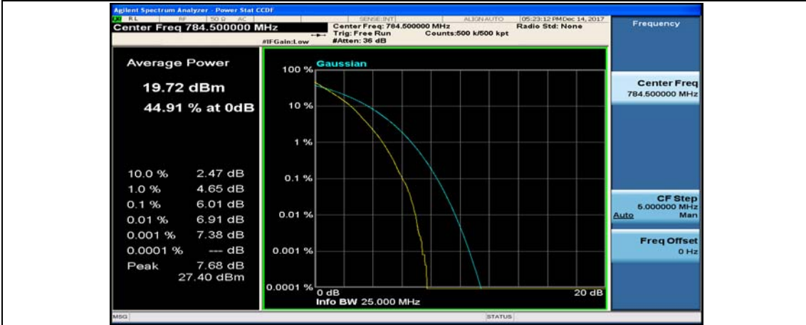
(Channel Bandwidth: 5 MHz)_HCH_QPSK_12RB#13
