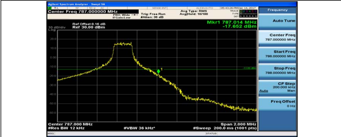
(Channel Bandwidth: 5 MHz)_HCH_QPSK_12RB#0
