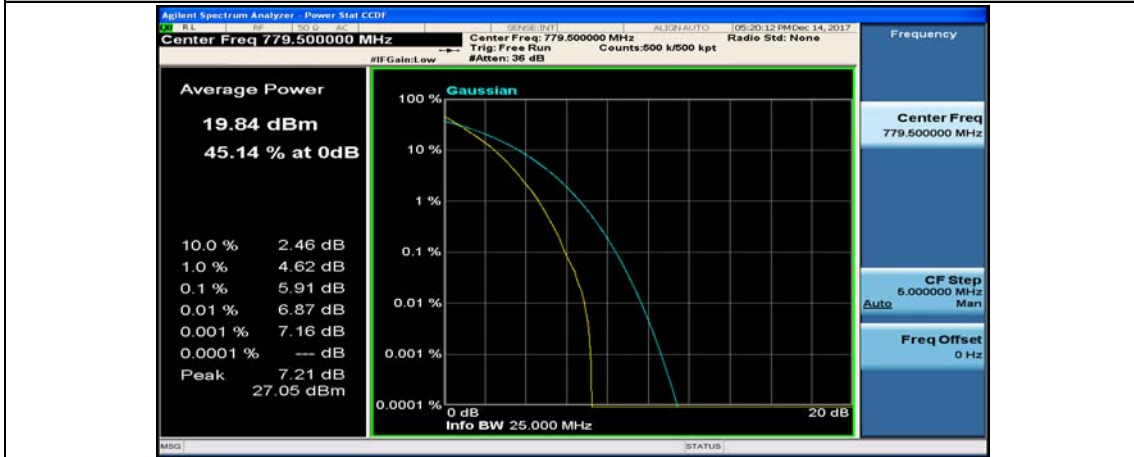
(Channel Bandwidth: 5 MHz)_LCH_QPSK_12RB#13
