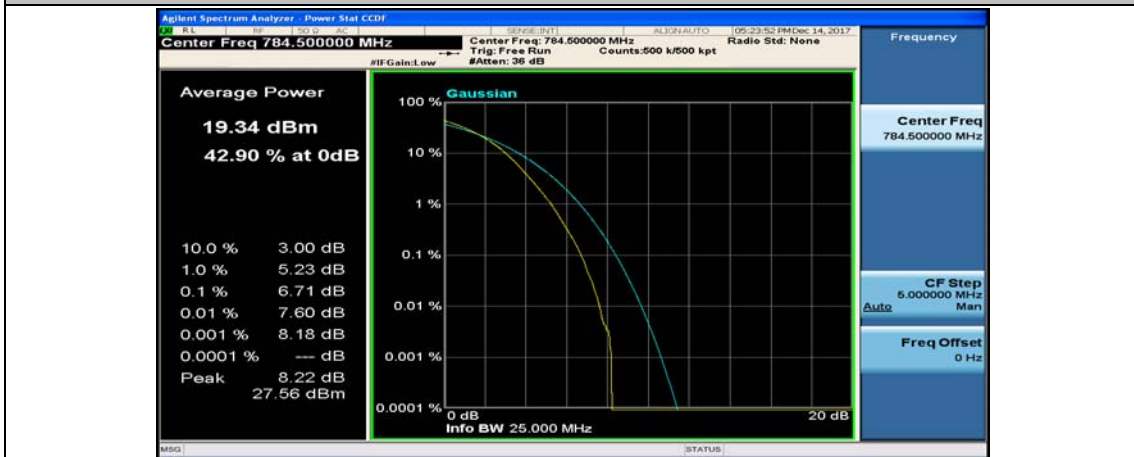
(Channel Bandwidth: 5 MHz)_HCH_16QAM_25RB#0
