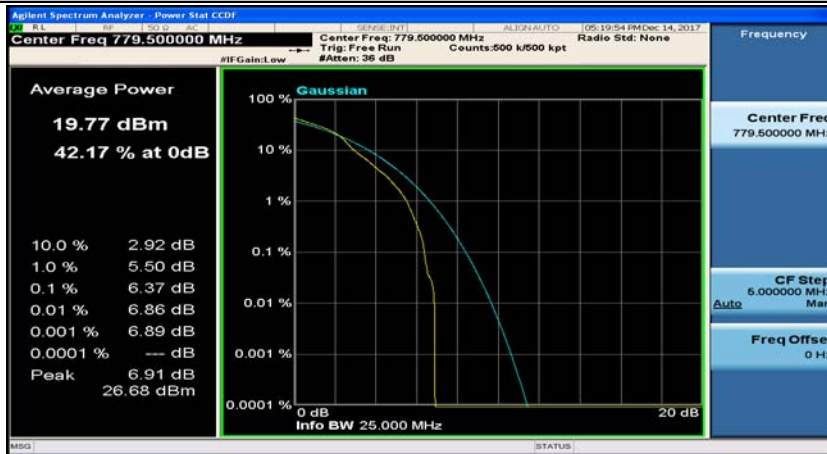
(Channel Bandwidth: 5 MHz)_LCH_16QAM_1RB#24
