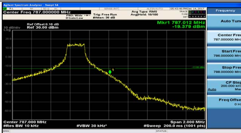
(Channel Bandwidth: 5 MHz)_HCH_16QAM_12RB#0
