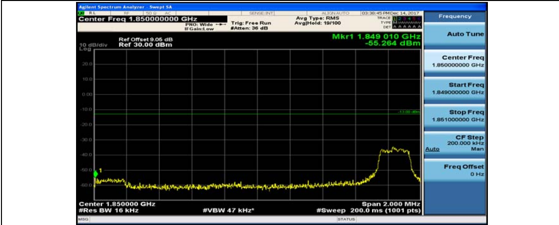
(Channel Bandwidth:15 MHz)_LCH_QPSK_37RB#0
