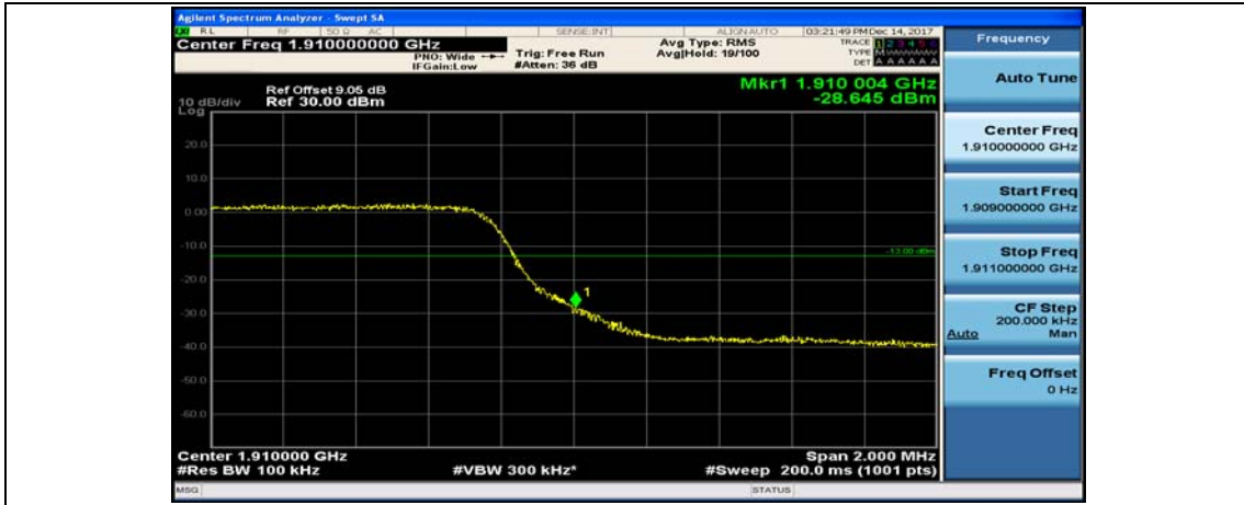
(Channel Bandwidth: 5 MHz)_LCH_16QAM_1RB#0
