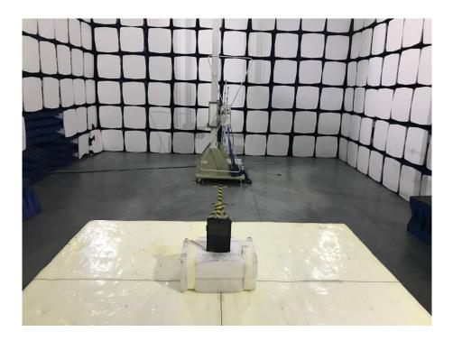
Radiation Emission Test Setup (1GHz to 18GHz)
