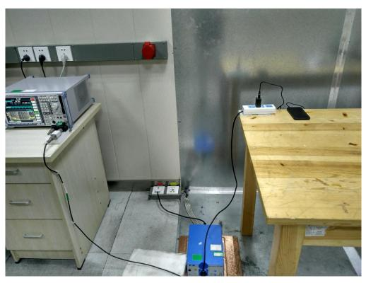
FCC RADIATED EMISSION TEST SETUP
