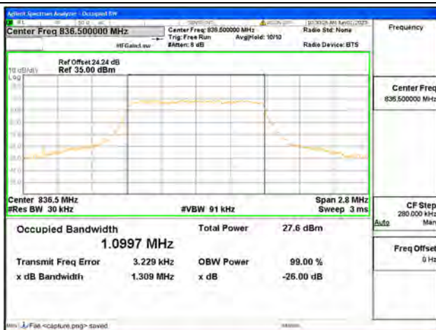
Band26 Part22 / 1.4MHz / 16QAM/ Mid CH
