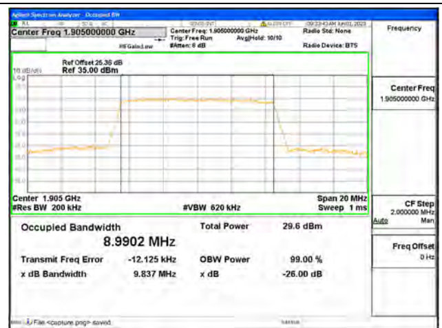
Band2 / 10MHz / QPSK/ High CH
