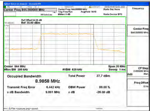
Band5 / 10MHz / QPSK/ High CH
