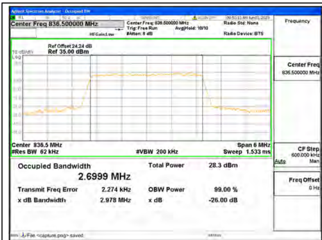
Band5 / 3MHz / QPSK/ Mid CH
