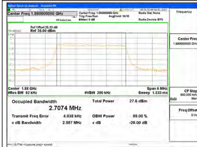
Band2 / 3MHz / 64QAM/ Mid CH
