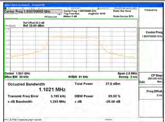
Band2 / 1.4MHz / 16QAM/ Low CH
