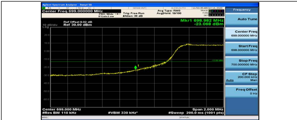
Channel Bandwidth: 10 MHz_LCH_QPSK_25RB#12
