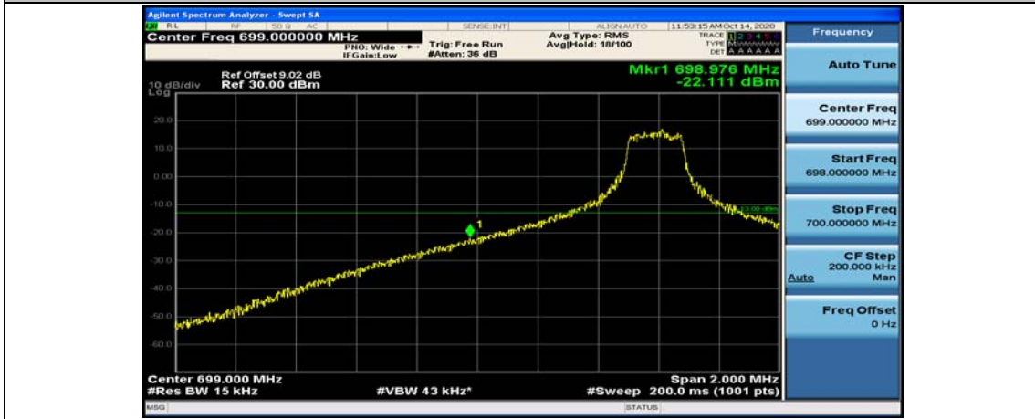
Channel Bandwidth: 10 MHz_LCH_16QAM_1RB#24
