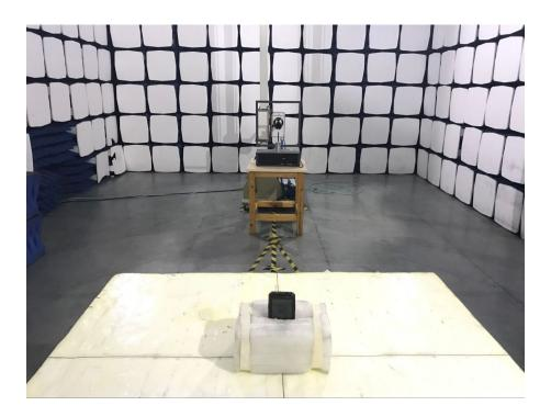
Radiation Emission Test Setup (30MHz to 1GHz)
