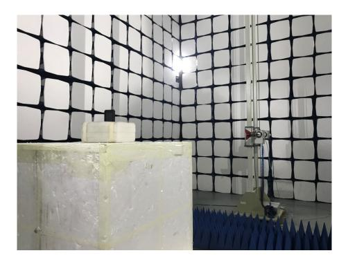
Radiation Emission Test Setup (Above 18GHz)
