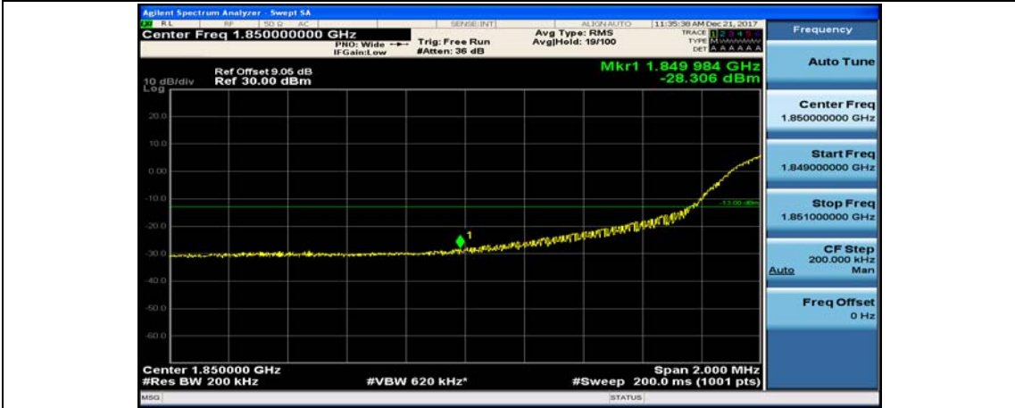
(Channel Bandwidth:20 MHz)_LCH_QPSK_50RB#25
