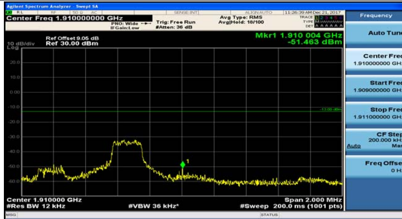
(Channel Bandwidth: 5 MHz)_HCH_QPSK_1RB#12
