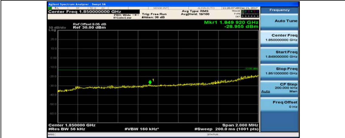
(Channel Bandwidth: 5 MHz)_LCH_16QAM_12RB#13
