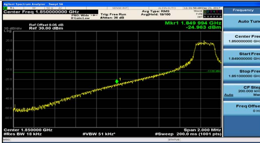
(Channel Bandwidth:15 MHz)_LCH_16QAM_1RB#37
