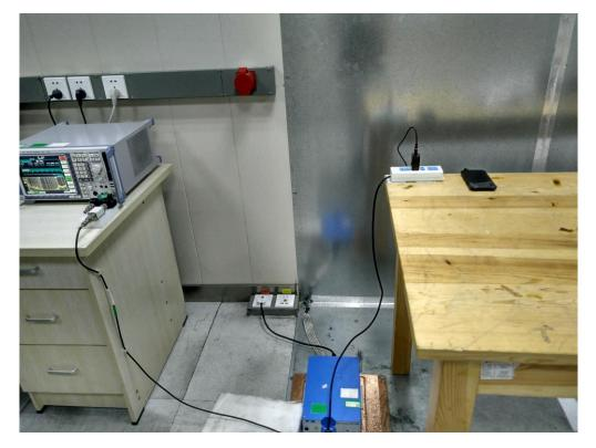
RADIATED EMISSION TEST SETUP
