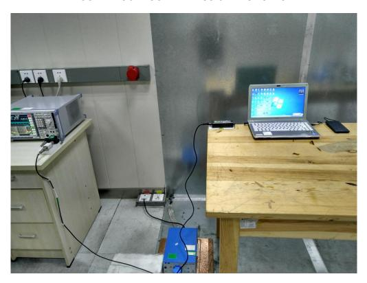
FCC RADIATED EMISSION TEST SETUP
