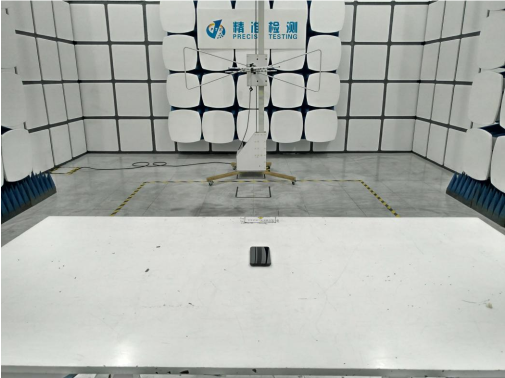
FCC RADIATED EMISSION TEST SETUP
