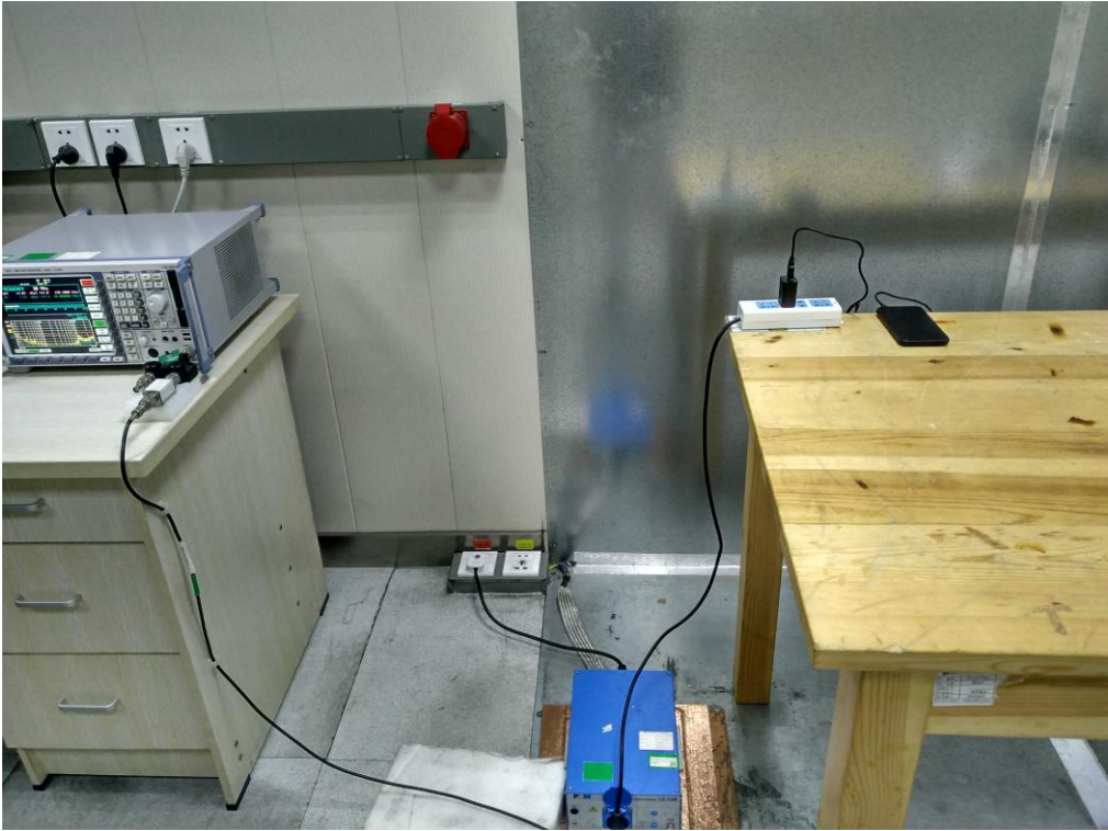
FCC RADIATED EMISSION TEST SETUP
