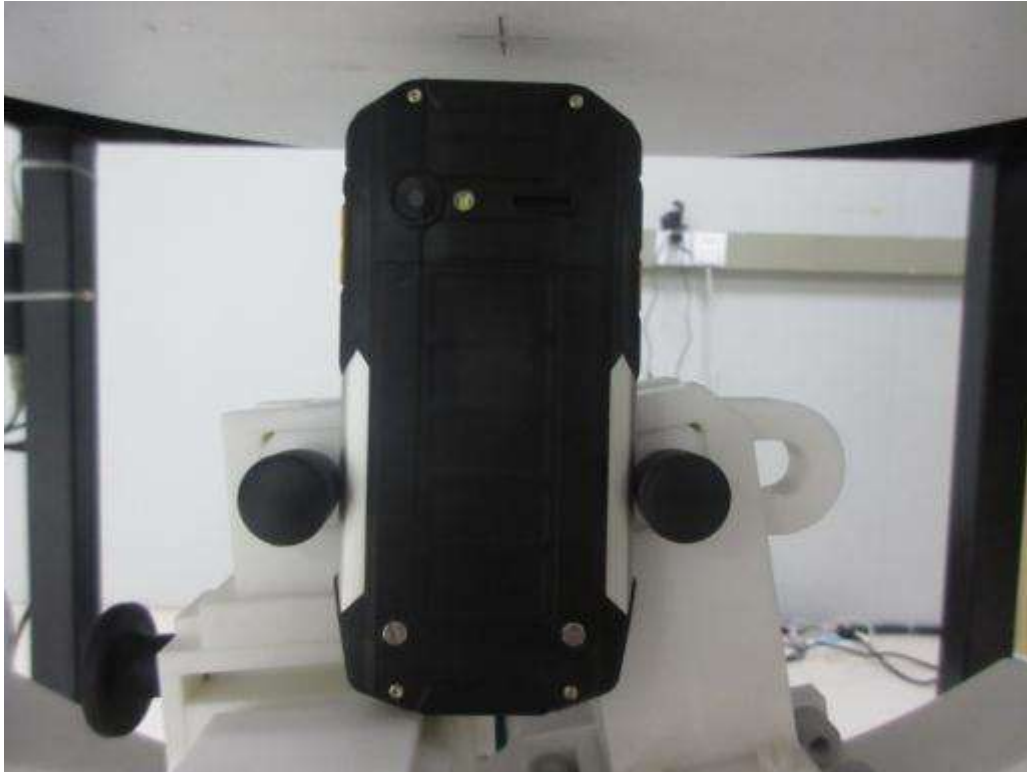
10mm body-worn Top Side Setup Photo(hotspot)
