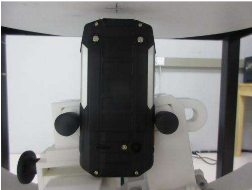
10mm body-worn Bottom Side Setup Photo(hotspot)
