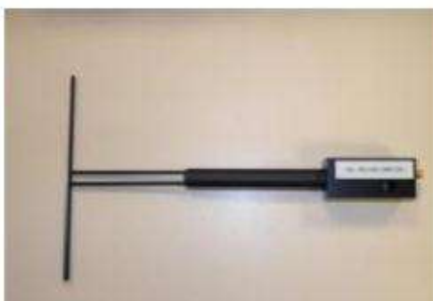
Figure 1 – Satimo COMOSAR Validation Dipole
