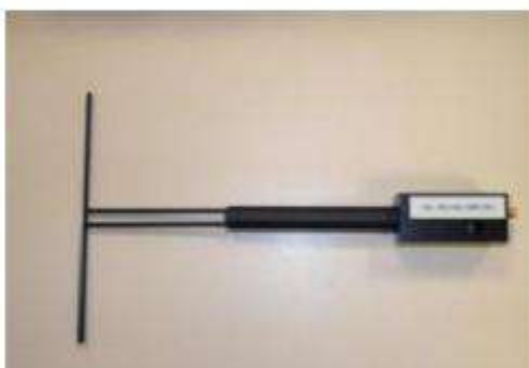
Figure 1 – Satimo COMOSAR Validation Dipole
