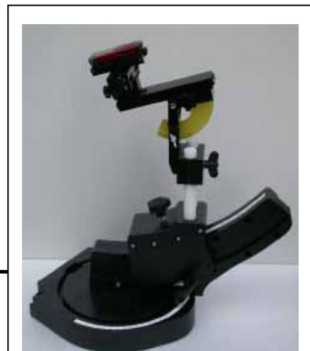
The DASY5 device holder has been made out of low-loss POM material having the following dielectric parameters: relative permittivity  $\epsilon_r = 3$  and loss tangent  $\delta = 0.02$ . The amount of dielectric material has been reduced in the closest vicinity of the device, since measurements have suggested that the influence of the clamp on the test results could thus be lowered.
