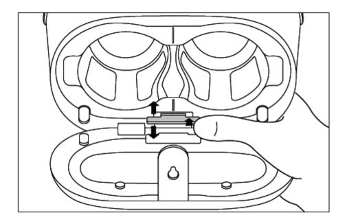
Adjust your mobile phone, and align the vertical line on the mobile phone with the line on the device.
