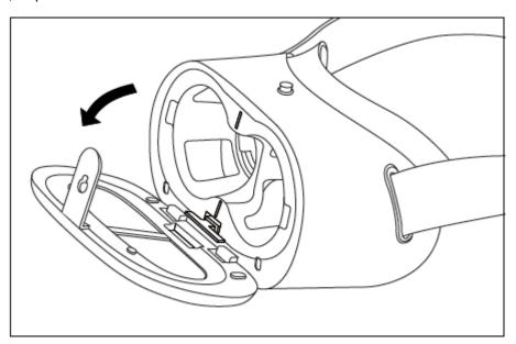
Adjust the gear (see picture) to a suitable position according to the size of your mobile phone. First gear matches 5 inch mobile phones, and third gear matches 6 inch mobile phones.
