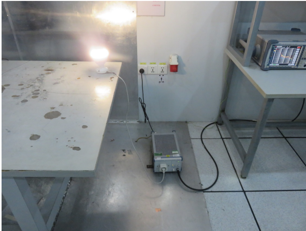
Photo of Radiation Emission Test
