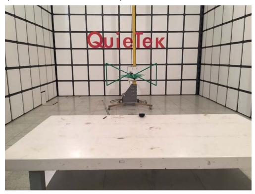
Description: Radiated Emission Test Setup for 1~18GHz
