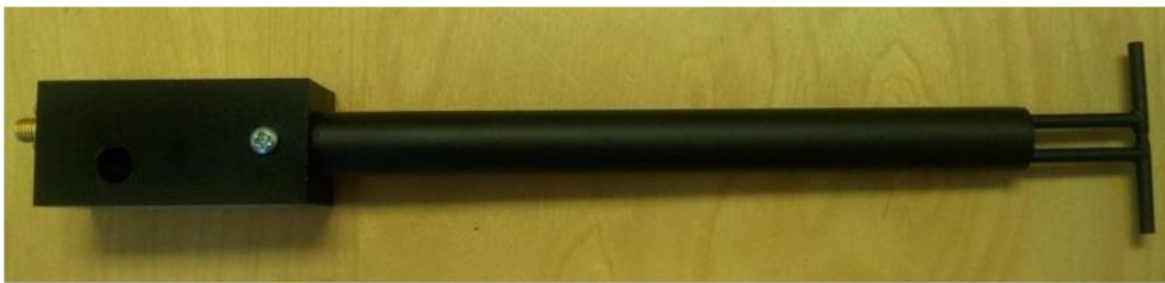
Figure 1 – MVG COMOSAR Validation Dipole
