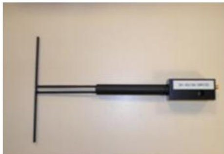
Figure 1 – Satimo COMOSAR Validation Dipole
