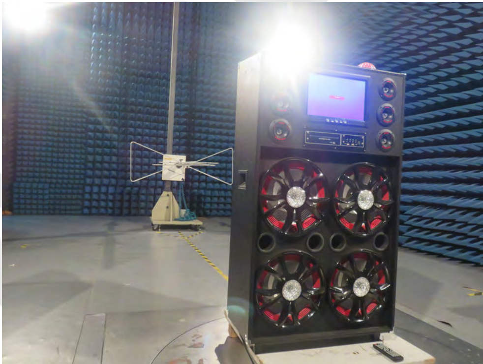
Photo of Radiation Emission Test
