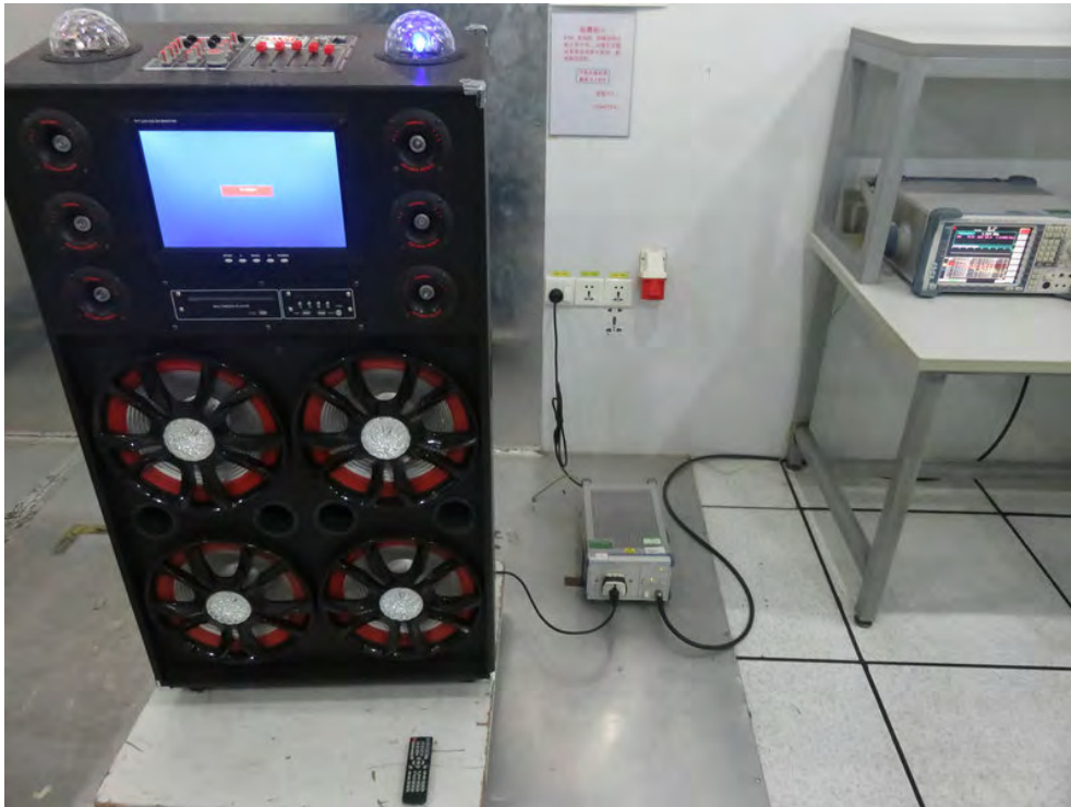
Photo of Conducted Emission Measurement
