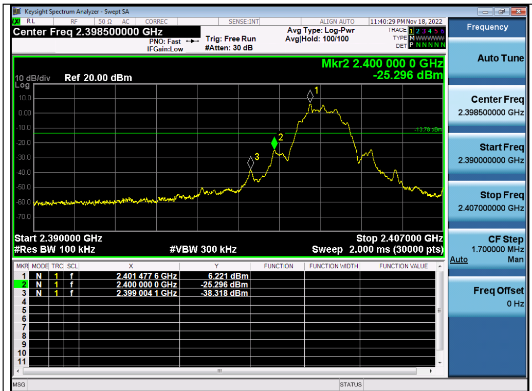
Test_Graph_LE2M_ANT1_2402_2Mbps_Lower Band Edge Emissions
