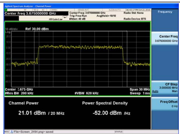
LTE Band 43 16QAM 20MHz CH44340
