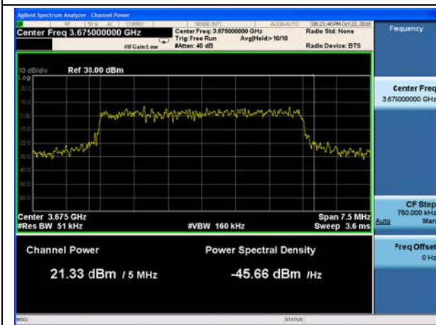
LTE Band 43 QPSK 5MHz CH44340
