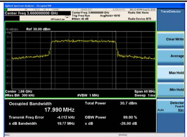
LTE Band 43 16QAM 20MHz CH44190
