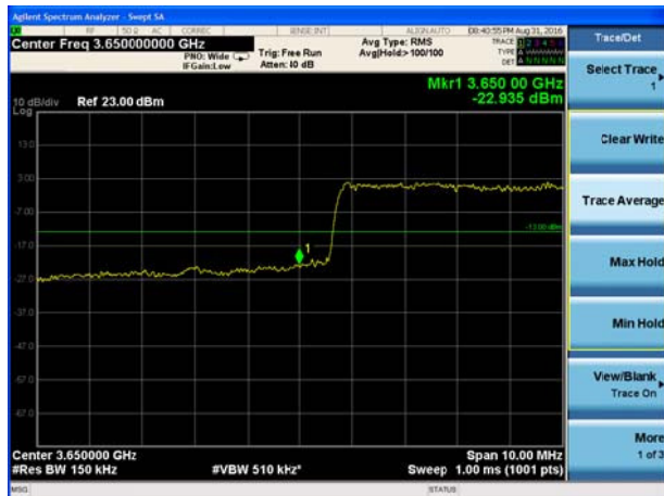
LTE Band 43 16QAM Bandwidth = 20MHz CH44190, RB 1
