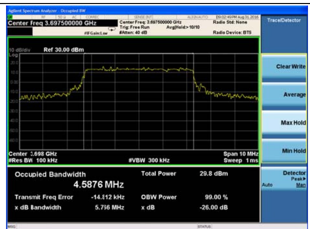
LTE Band 43 16QAM 5MHz CH44565
