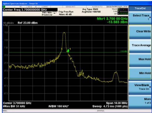
LTE Band 43 QPSK Bandwidth = 5MHz CH44565, RB 25
