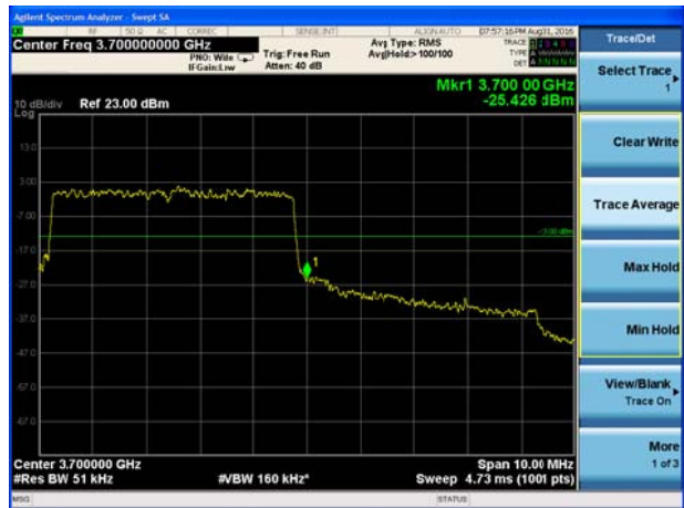
LTE Band 43 QPSK Bandwidth = 10MHz CH44540, RB 1
