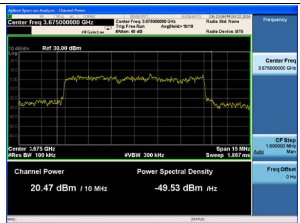
LTE Band 43 16QAM 10MHz CH44340
