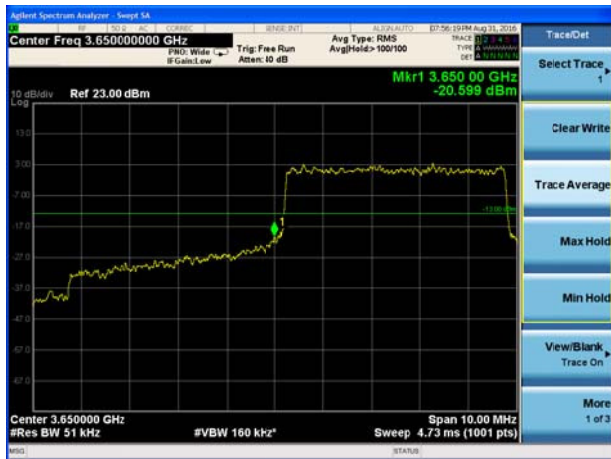
LTE Band 43 QPSK Bandwidth = 10MHz CH44140, RB 1
