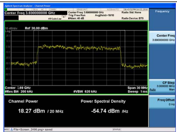
LTE Band 43 16QAM 20MHz CH44490
