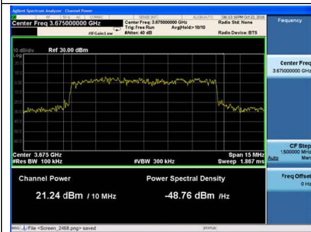
LTE Band 43 QPSK 10MHz CH44340
