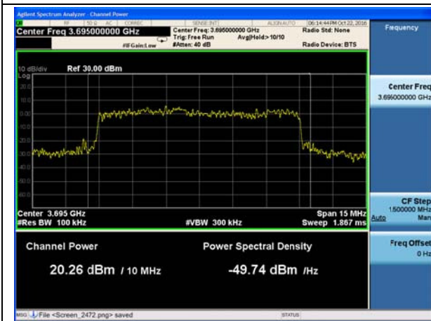
LTE Band 43 QPSK 10MHz CH44540
