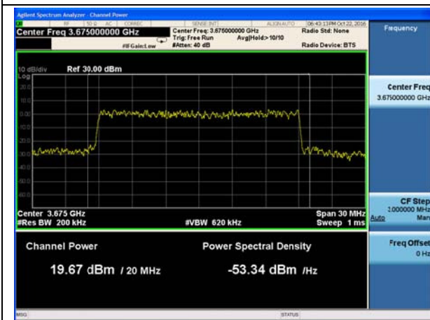
LTE Band 43 QPSK 20MHz CH44340
