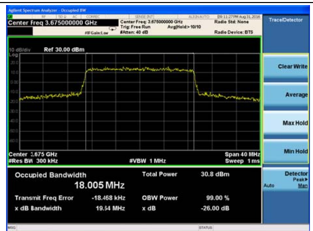
LTE Band 43 16QAM 20MHz CH44340
