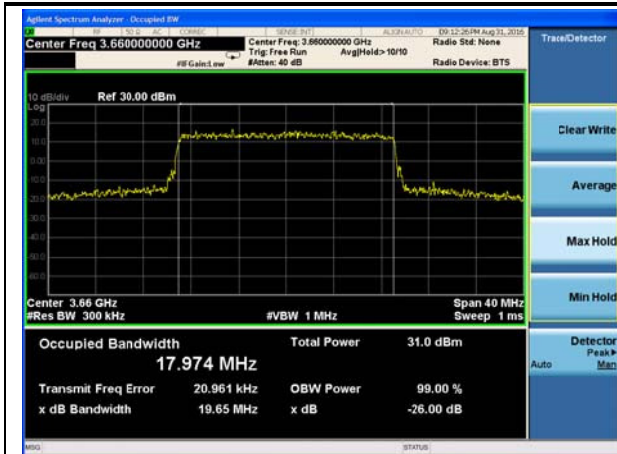
LTE Band 43 QPSK 20MHz CH44190
