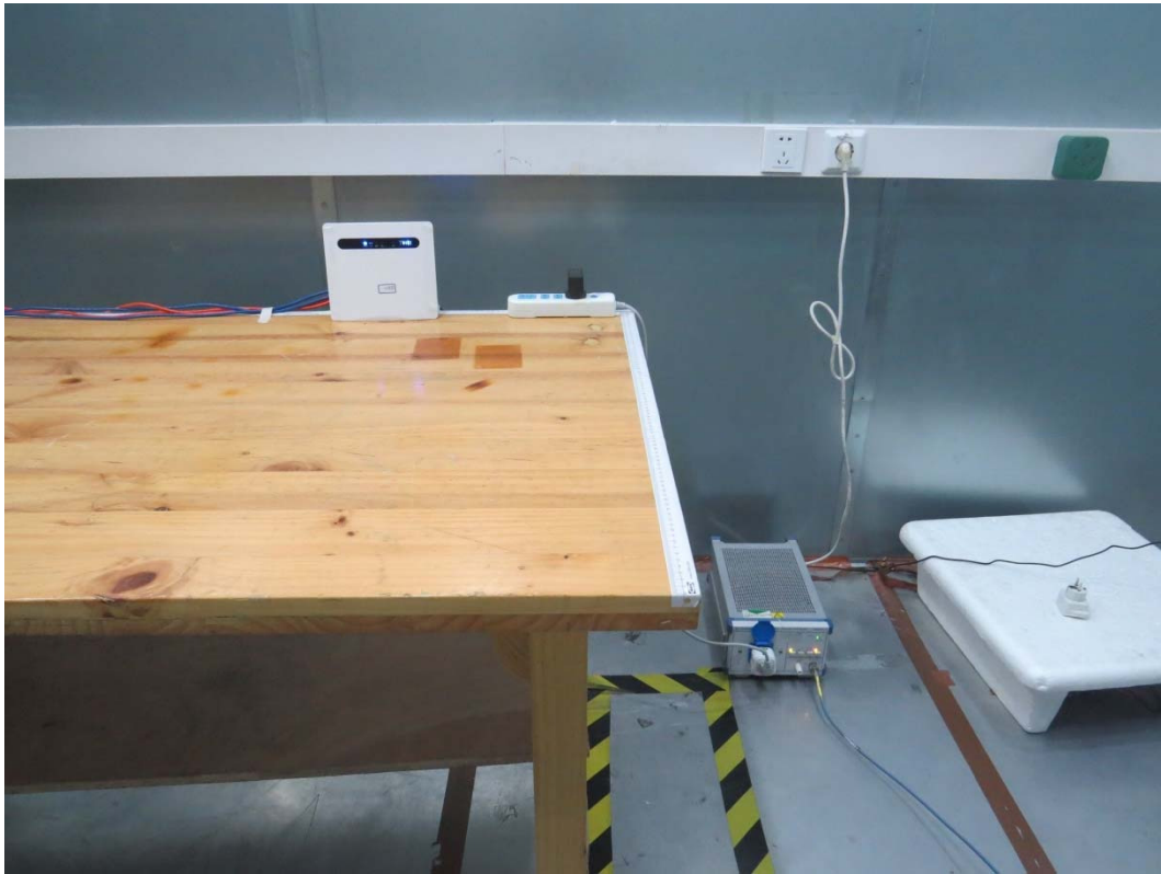
Picture 3 Conducted Emission Test Setup
