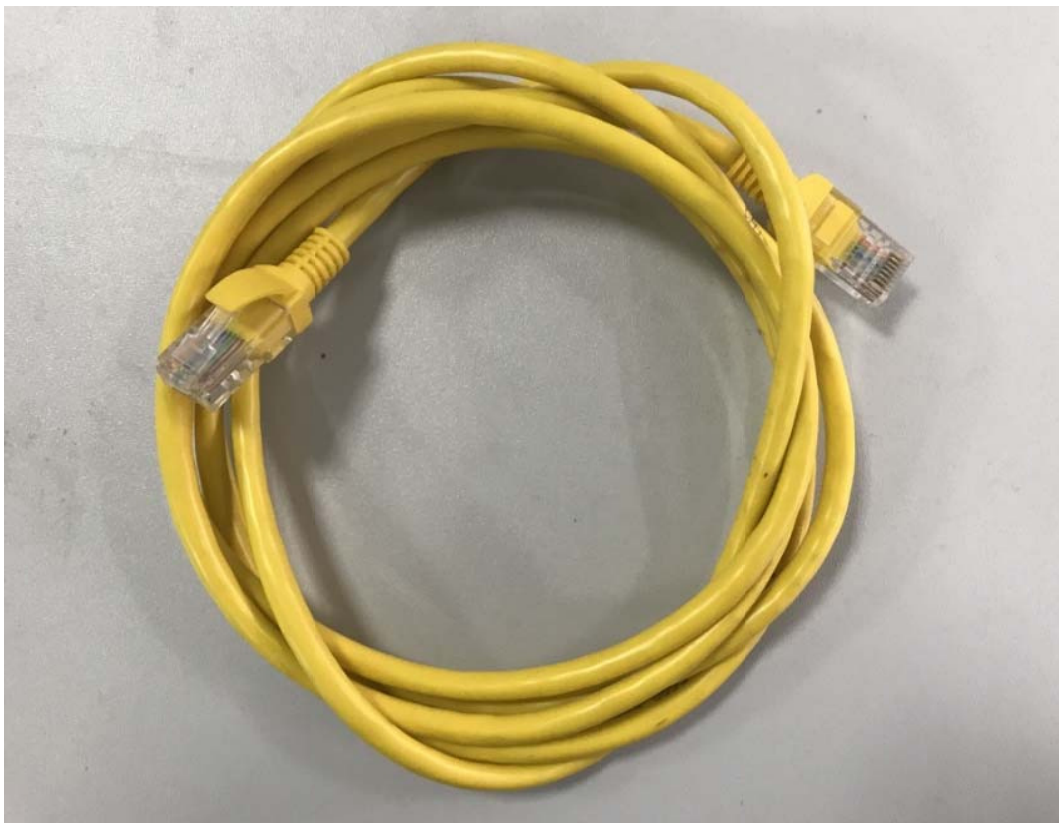
c: Ethernet cables
