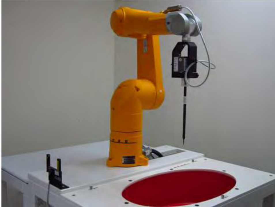
Fig.1 Photograph of the SAR measurement system
