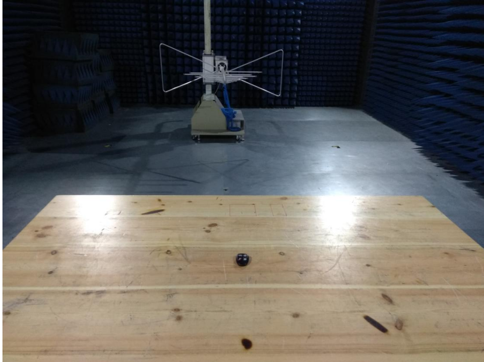
Photo of Radiated Emission Measurement
