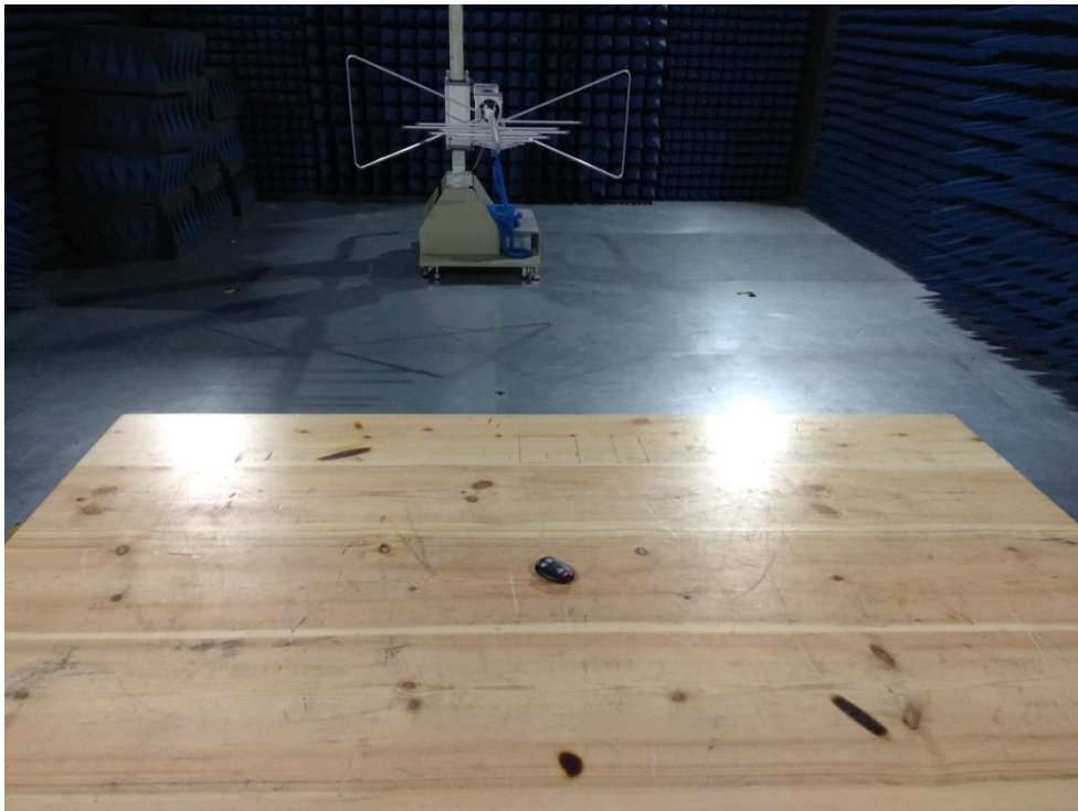
Photo of Radiated Emission Measurement
