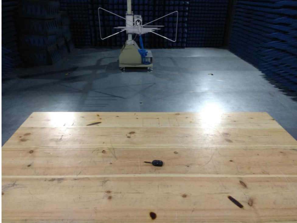
Photo of Radiated Emission Measurement
