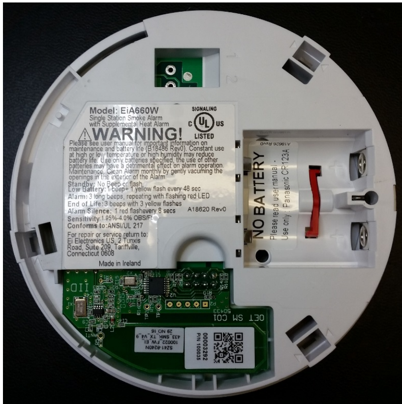
Internal with radio installed
