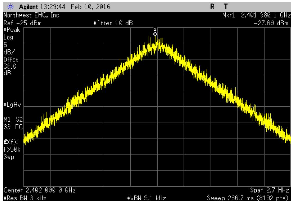
2400 MHz - 2483.5 MHz Band, Zigbee GFSK, Mid Channel 40, 2440 MHz
