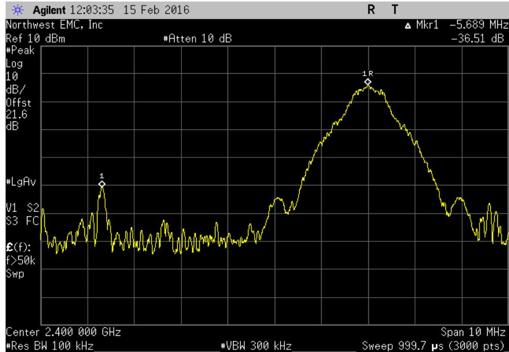
Normal Temperature Conditions, Zigbee GFSK, High Channel, 81, 2481 MHz
