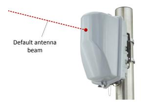
The orientation of the StreetNode<sup>TM</sup> 6250 PTP antenna is not critical as node has self-alignment capabilities with tilt range  $30^{\circ}$  (±15°) and elevation range  $20^{\circ}$  (±10°).
