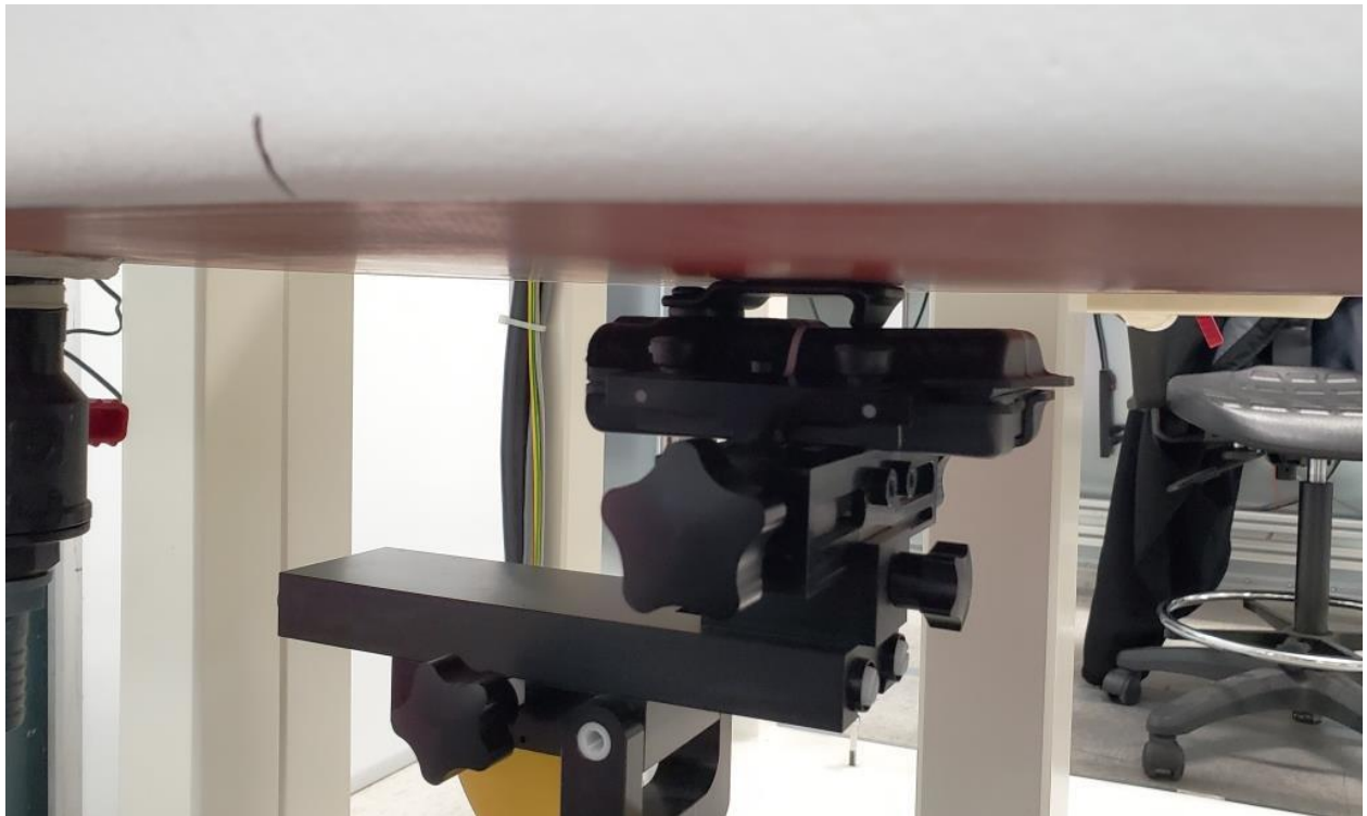
EUT with holster clip against flat area of phantom with 0mm spacing
