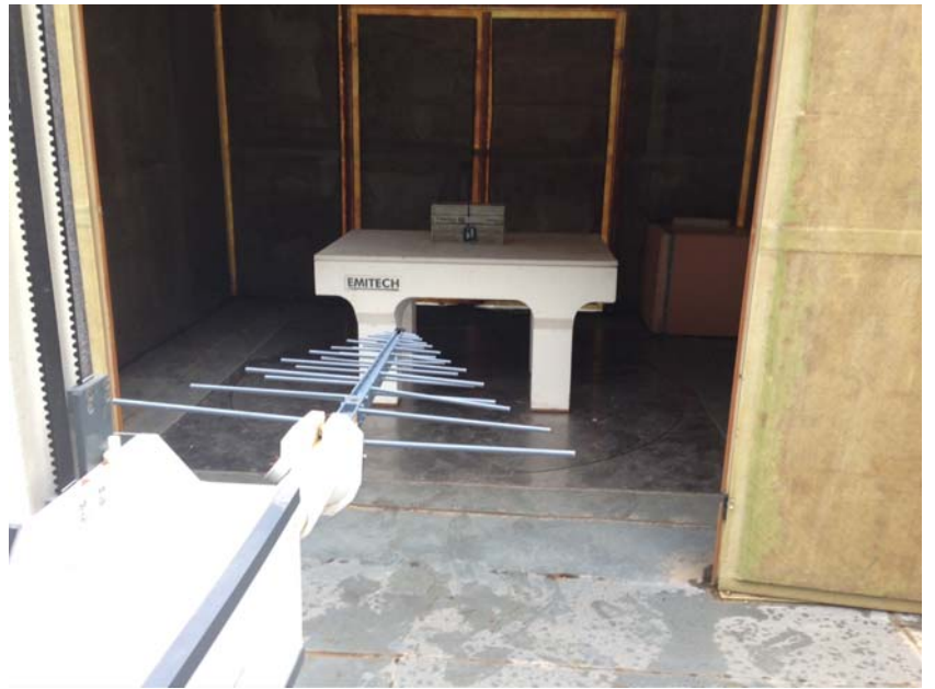
Open area test site measurement
