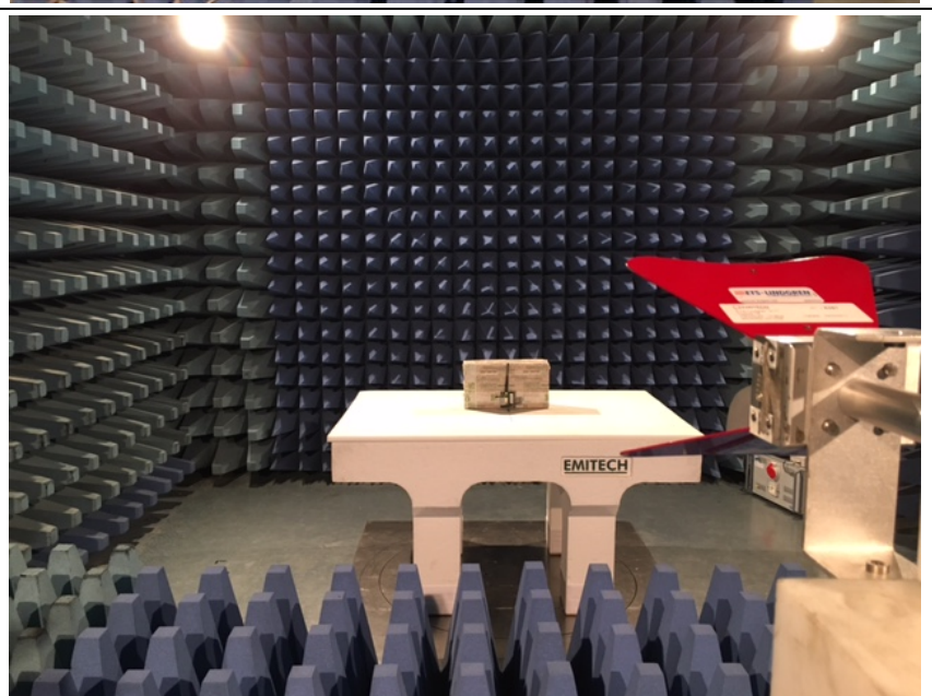
Radiated electric field in anechoic chamber (f>1GHz)
