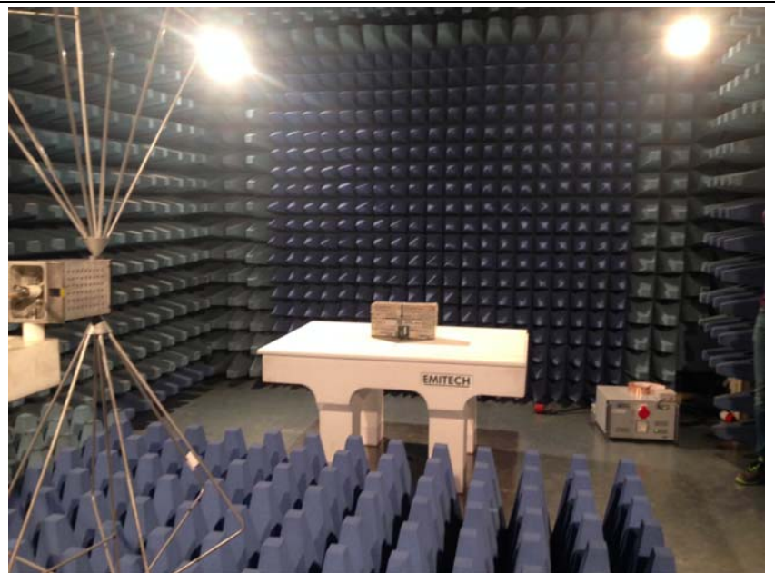
Radiated electric field in anechoic chamber
