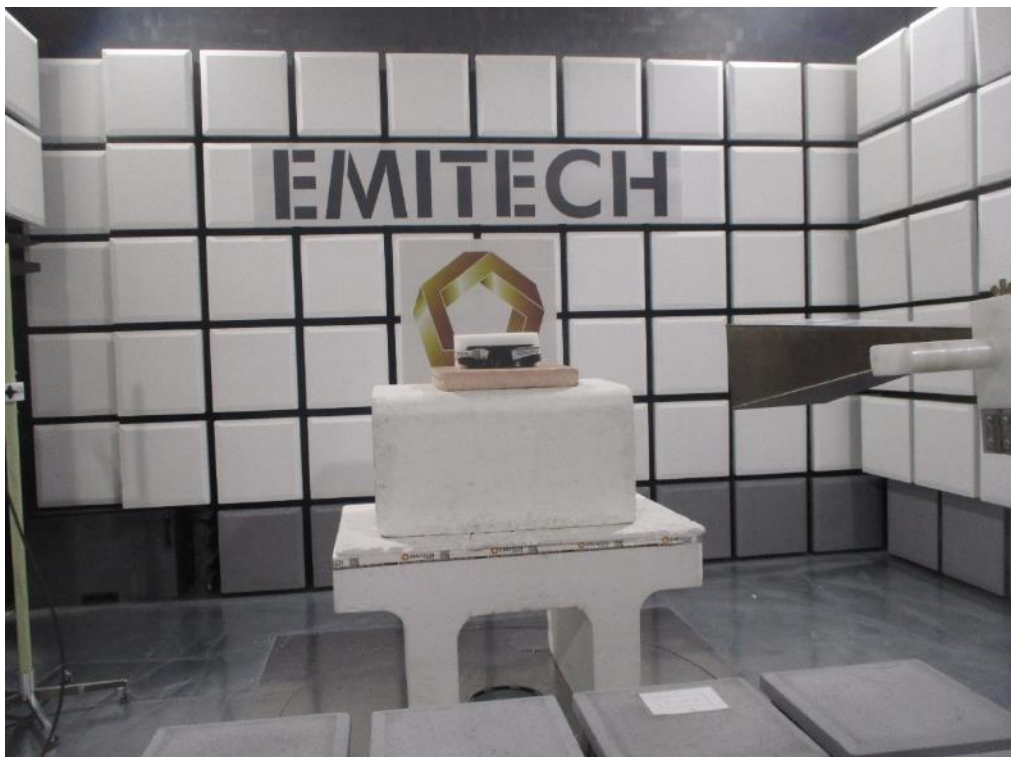
TEST SETUP PHOTO - 18GHZ – 25GHZ
