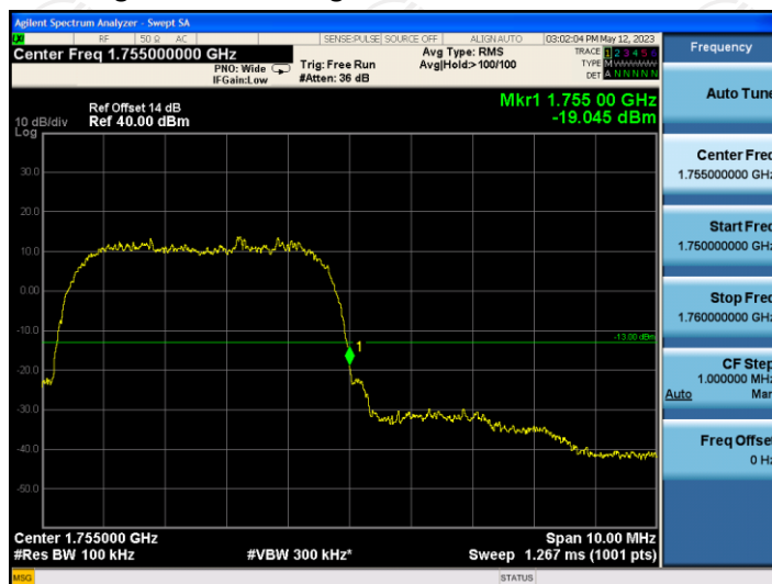
Higher Band Edge Plot on Channel 1513
