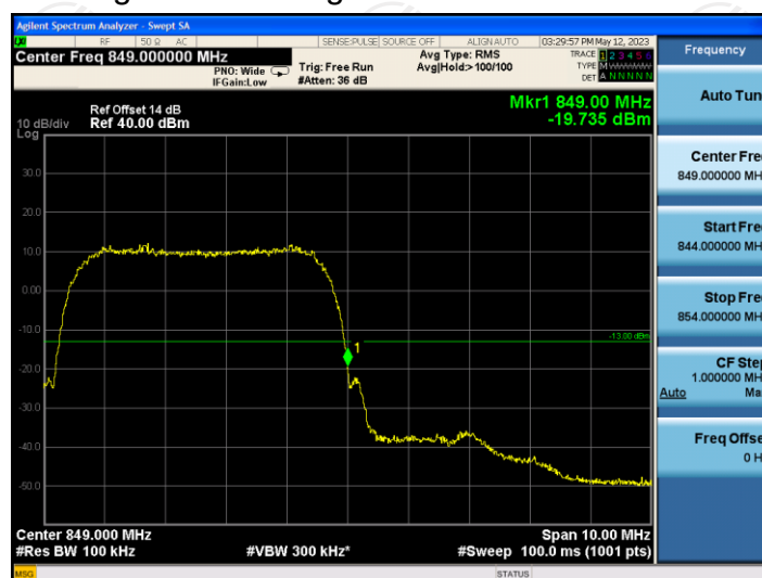
Higher Band Edge Plot on Channel 4233
