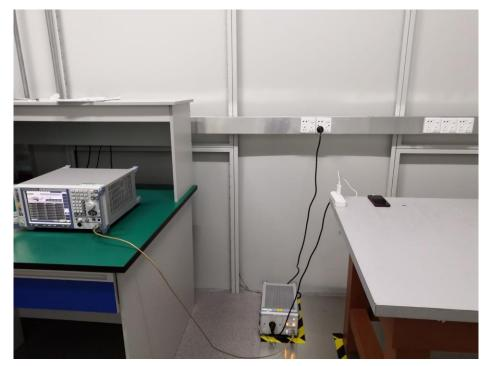
RADIATED EMISSION TEST SETUP
