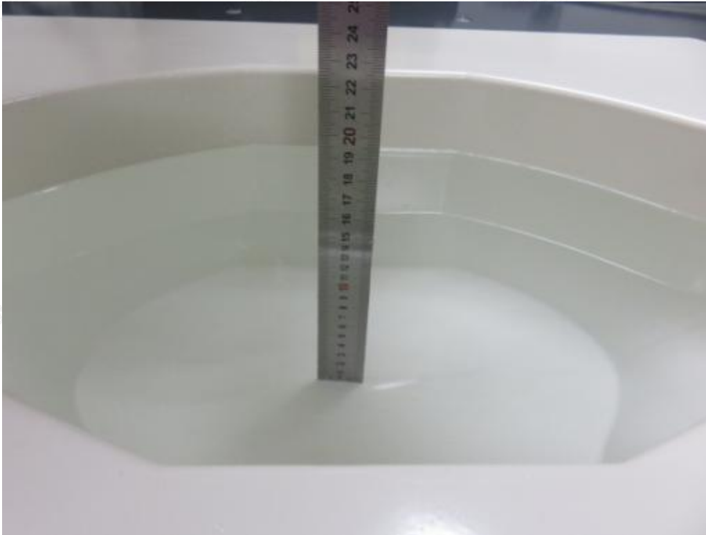
Photograph of the depth in the Head Phantom (1800MHz, 16.1cm depth)
