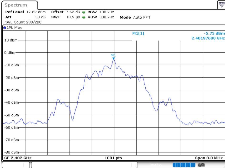
Band Edge NVNT GFSK 2402MHz Ant1 Emission
