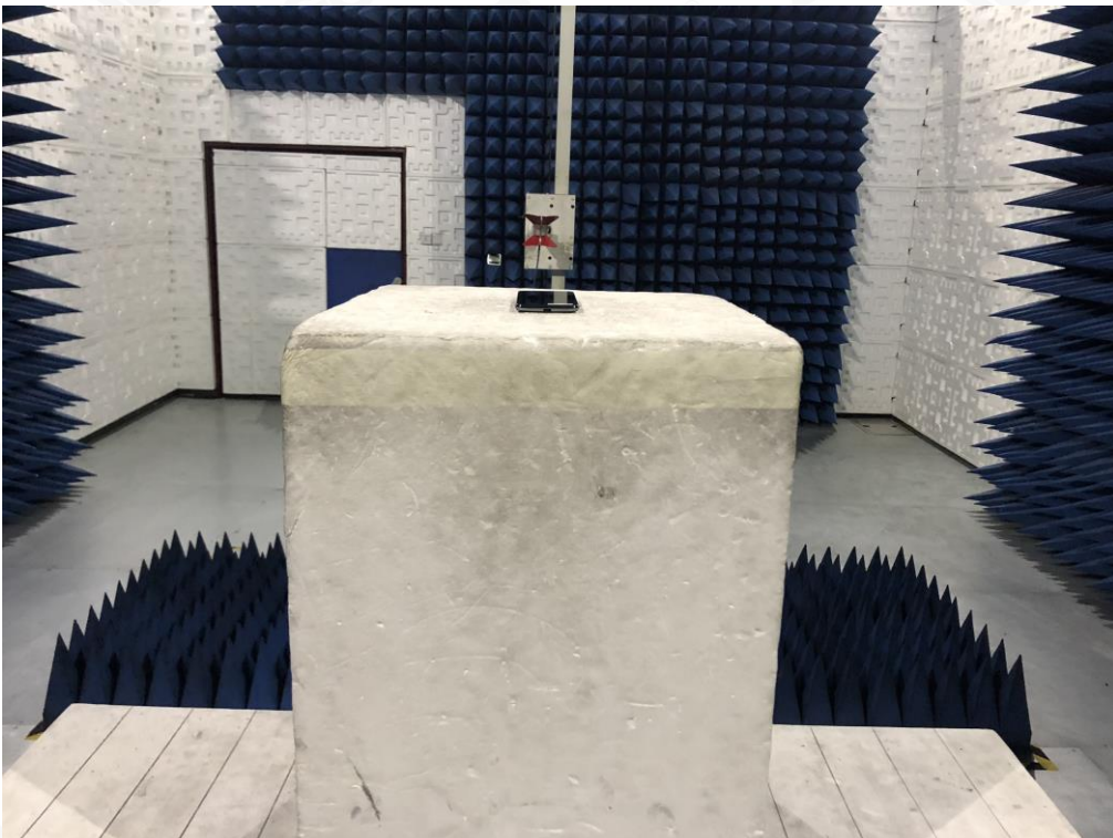
RADIATED EMISSION TEST SETUP ABOVE 1GHZ
