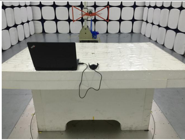
Radiated Spurious Emissions Test Setup Below 1GHz
