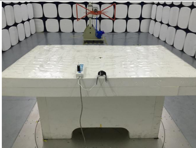
Radiated Emissions Test Setup Below 1GHz
