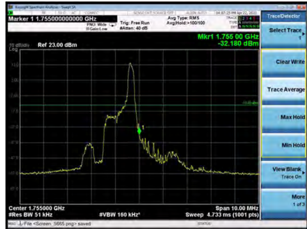
LTE Band 4 QPSK 5MHz CH-High, 100%RB
