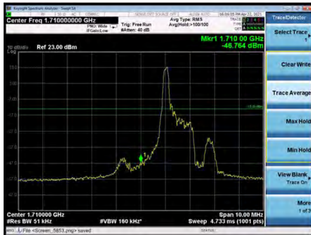
LTE Band 66 16QAM 15MHz CH-Low, 1 RB
