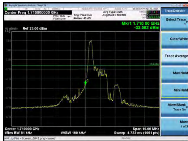
LTE Band 66 QPSK 5MHz CH-Low, 100%RB
