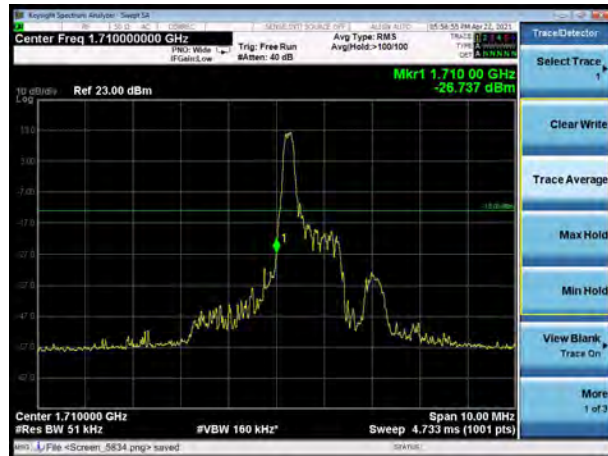
LTE Band 66 16QAM 1.4MHz CH-Low, 100%RB
