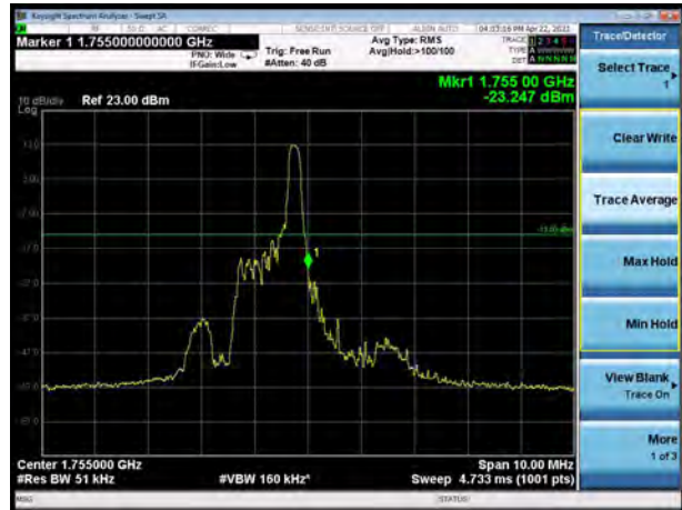
LTE Band 4 QPSK 1.4MHz CH-High, 100%RB
