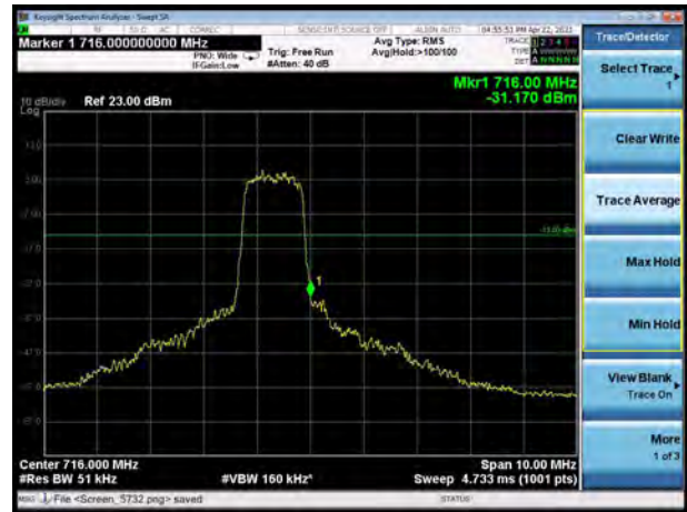
LTE Band 12 16QAM 3MHz CH-High, 1 RB
