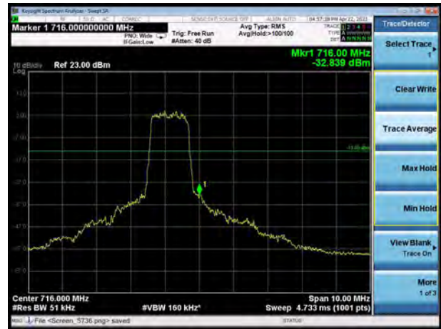
LTE Band 12 16QAM 3MHz CH-High, 100%RB
