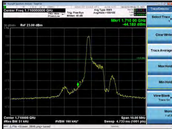
LTE Band 66 16QAM 10MHz CH-Low, 100%RB
