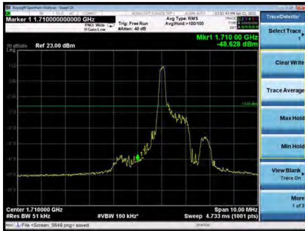
LTE Band 4 QPSK 15MHz CH-Low, 1 RB
