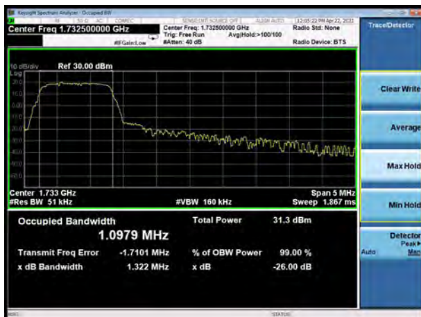
LTE Band 4 QPSK 5MHz CH-Middle
