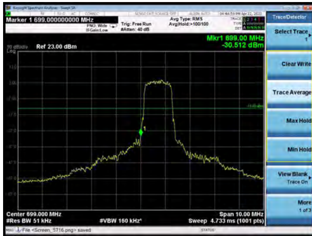
LTE Band 12 16QAM 3MHz CH-Low, 1 RB
