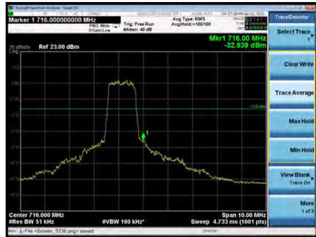
LTE Band 12 QPSK 5MHz CH-High, 1 RB
