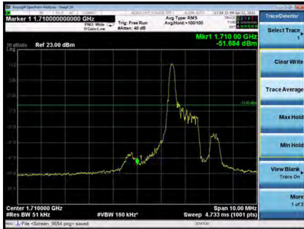
LTE Band 4 16QAM 20MHz CH-Low, 100%RB
