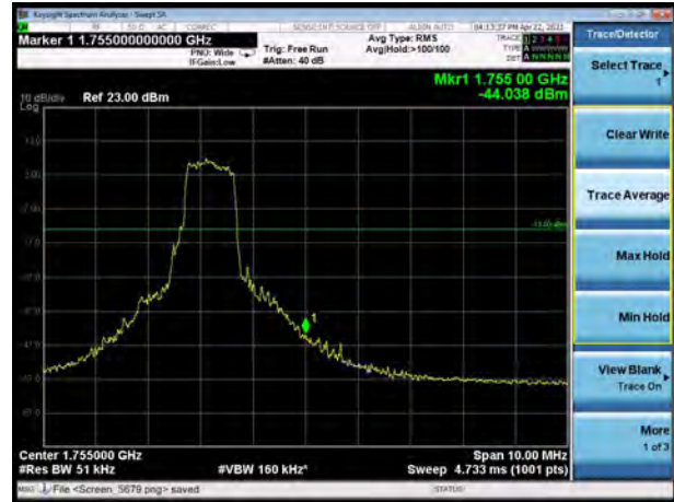
LTE Band 4 16QAM 20MHz CH-High, 100%RB
