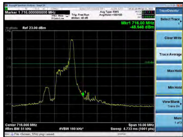
LTE Band 12 16QAM 10MHz CH-High, 1 RB
