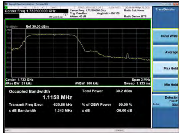
LTE Band 4 QPSK 10MHz CH-Middle
