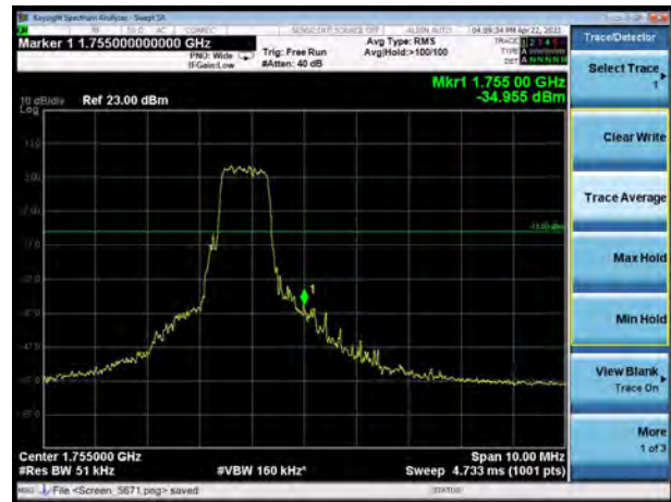
LTE Band 4 16QAM 15MHz CH-High, 1 RB
