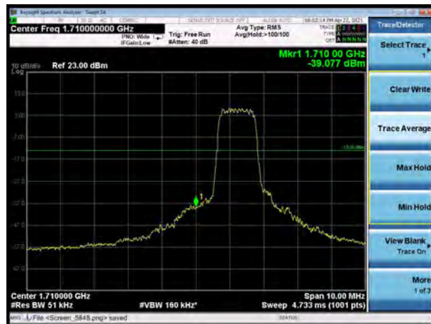
LTE Band 66 QPSK 15MHz CH-Low, 1 RB
