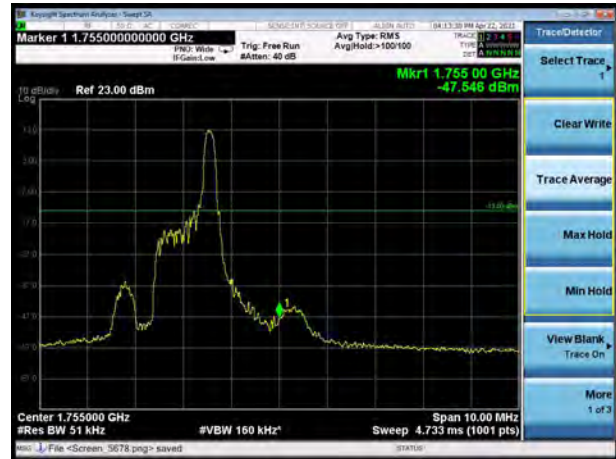
LTE Band 4 16QAM 20MHz CH-High, 100%RB
