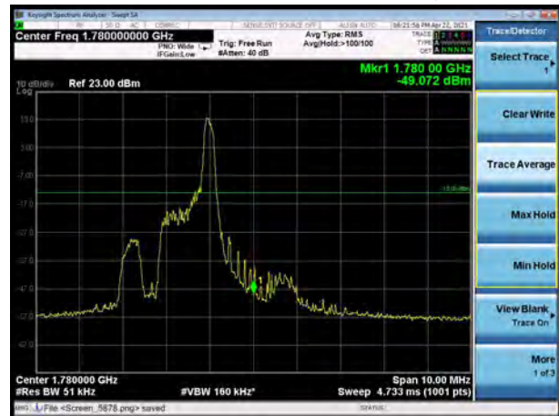
LTE Band 66 QPSK 15MHz CH-High, 1 RB
