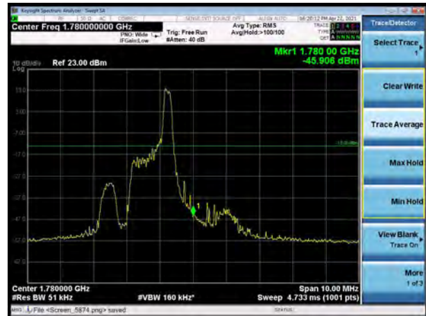
LTE Band 66 QPSK 10MHz CH-High, 100%RB
