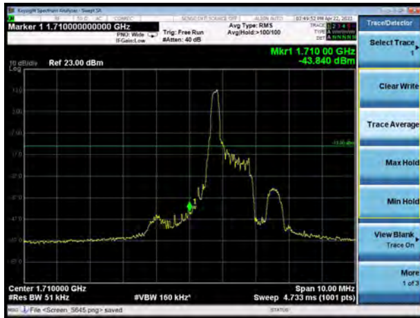
LTE Band 4 QPSK 10MHz CH-Low, 100%RB
