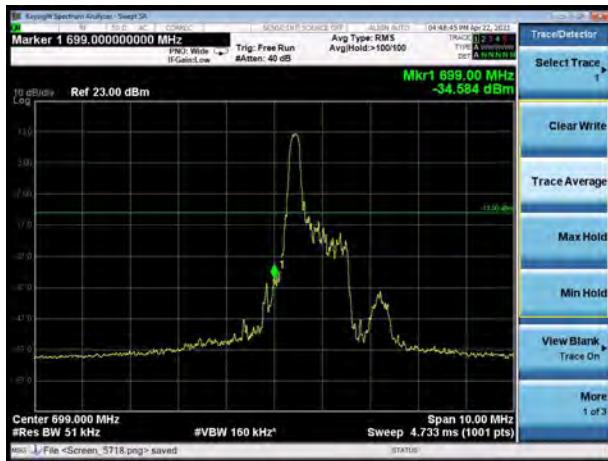
LTE Band 12 16QAM 3MHz CH-Low, 100%RB
