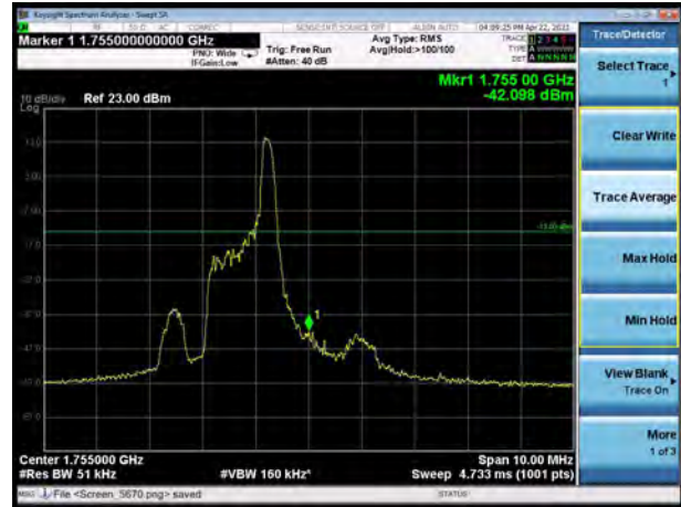
LTE Band 4 16QAM 10MHz CH-High, 100%RB
