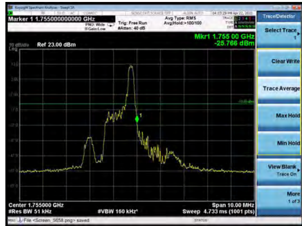
LTE Band 4 16QAM 1.4MHz CH-High, 100%RB
