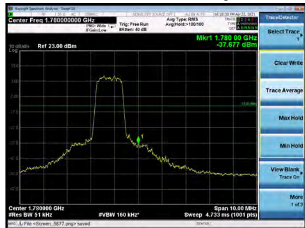
LTE Band 66 QPSK 15MHz CH-High, 1 RB
