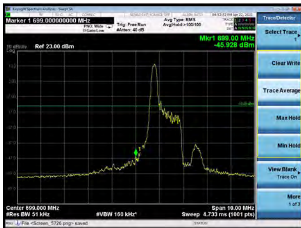
LTE Band 12 16QAM 10MHz CH-Low, 1 RB
