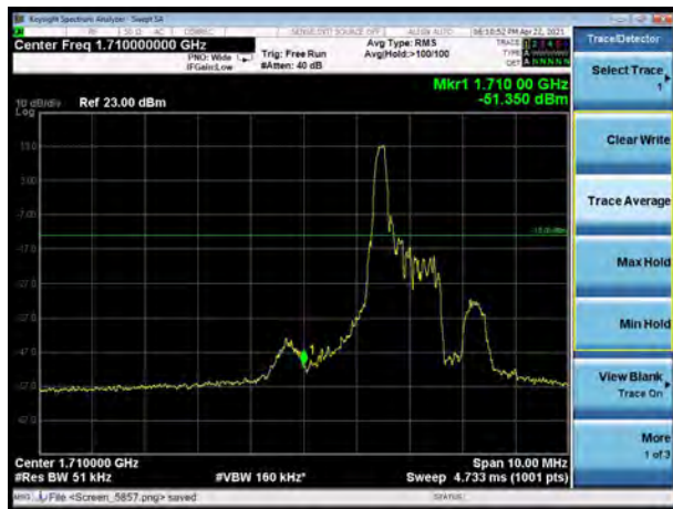
LTE Band 66 16QAM 20MHz CH-Low, 100%RB
