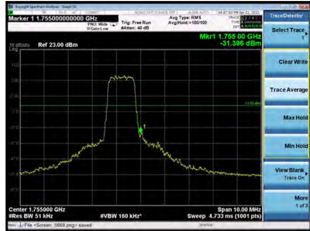
LTE Band 4 QPSK 5MHz CH-High, 100%RB
