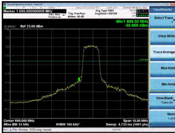
LTE Band 12 QPSK 5MHz CH-Low, 1 RB
